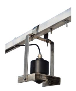
Non-Contact Water Level sensor (Radar Type) used to monitor the water level of surface water, dams, lakes, pools, aquatic ponds. This sensor can be connected to data-logger, controller or to some display by means of electronic interface.
